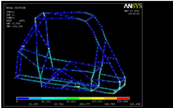
Fig 8. Von mises stress diagram.
