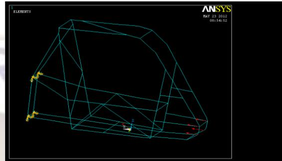
Fig 5. Applied load and displacement.
