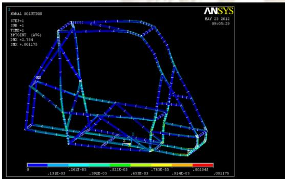
Fig 9. Total mechanical strain intensity diagram for rollage.
