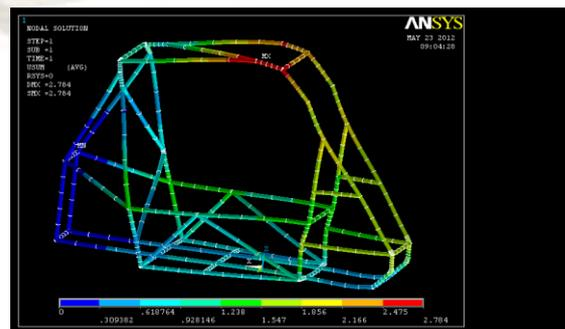
Fig 7. Nodal displacement diagram of the rollage.
