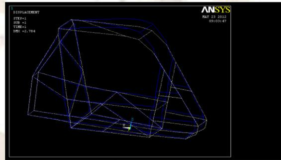
Fig 6. Deformed shape of the rollage.
