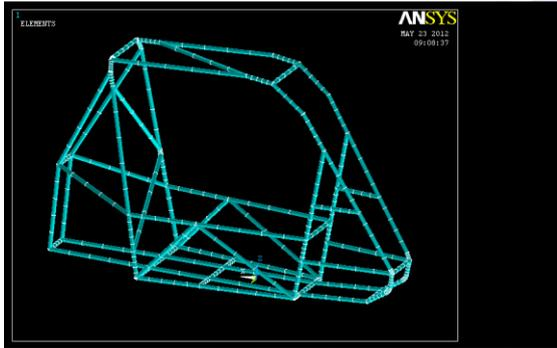
Fig 4. Meshed model with element shape.
